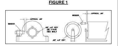
Note: When mounting sensor on small idler rollers (less than 6 inches in diameter), install a <u>maximum</u> of 2 targets
